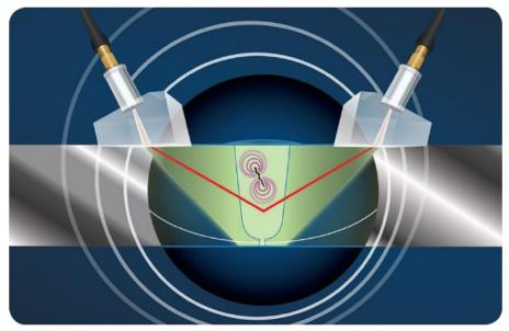
Time of Flight Diffraction (ToFD)
